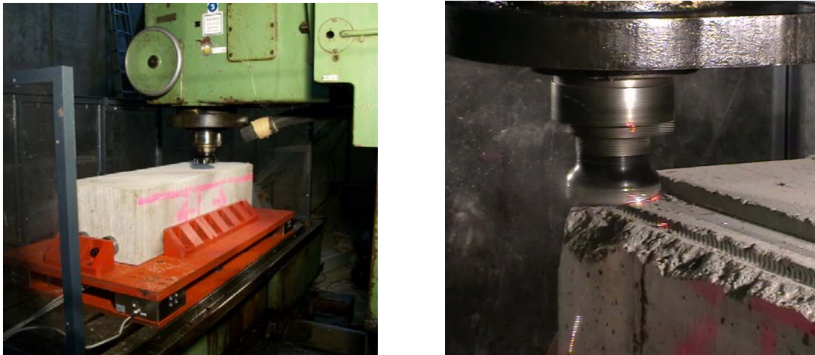
Figure 4: Ablation test bench for milling tests
