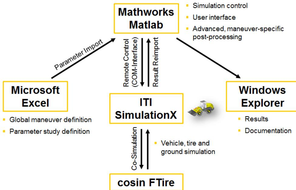
Figure 1: Tool chain of the automated simulation process
