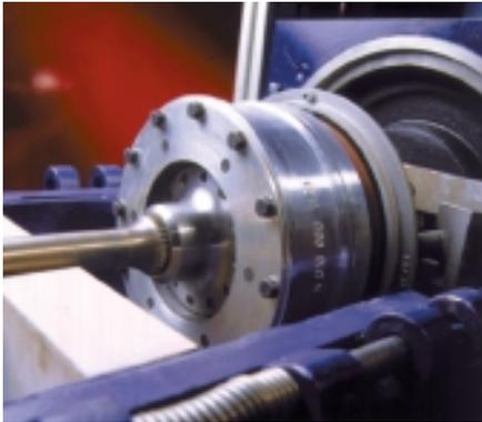
Fig. 5: T10F installed with damping element and flexible connection shaft
