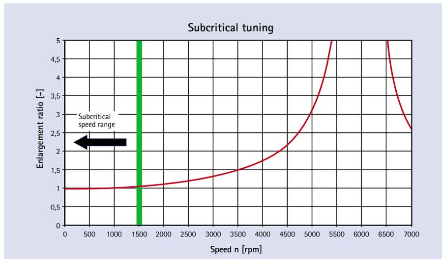
Fig. 8: Operating range for the subcritical design
