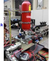
A central aspect of the work is the reliable control of oil temperature and pressure, ensuring both parameters can be adjusted to defined values. The flow rate through the crack must be measured accurately. The thesis therefore includes conceptual planning, designing the final system, assembly, and the execution of initial measurement series to verify functionality and measurement accuracy.
