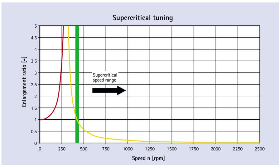
Fig. 7: Operating range for the supercritical design
