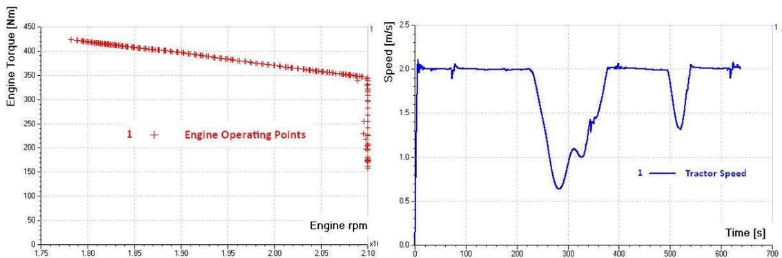
Figure 7. Engine Operating Points and Tractor Speed
