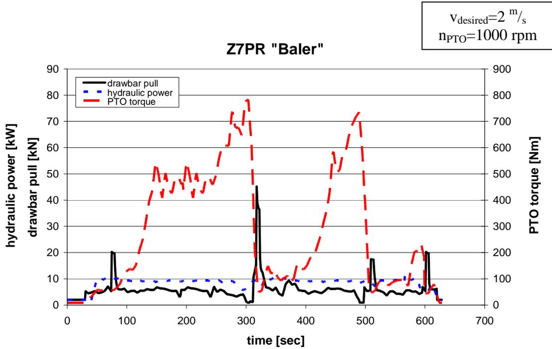
Figure 6. PowerMix Cycle Z7PR (according to [25])
