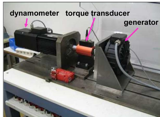
**Fig. 2. Test bench for determination of characteristic maps**
