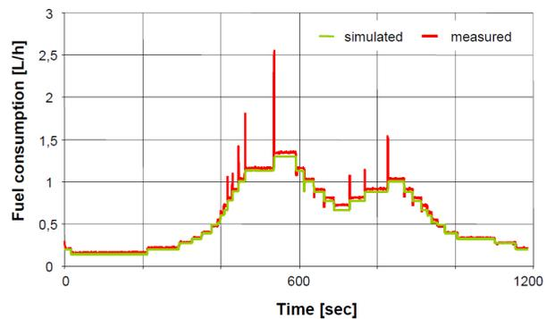
Fig. 8. Time dependent fuel consumption, simulation and test results
