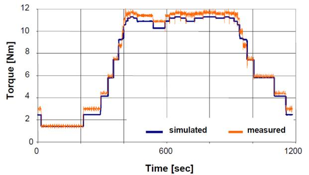
Fig. 7. Time dependent diesel torque, simulation and test results
