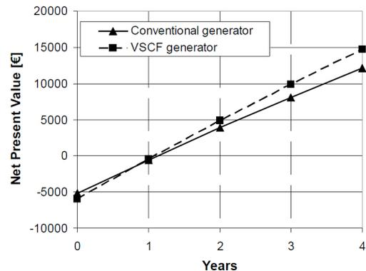
**Fig. 10. Net present value evolution of a VSCF generator and a constant speed generator**
