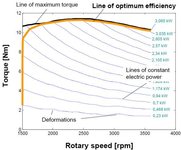
**Fig. 3. Determined characteristic curve of optimum fuel consumption of the system**
