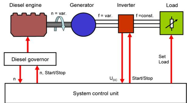
**Fig. 1. Set up of the analysed system**
