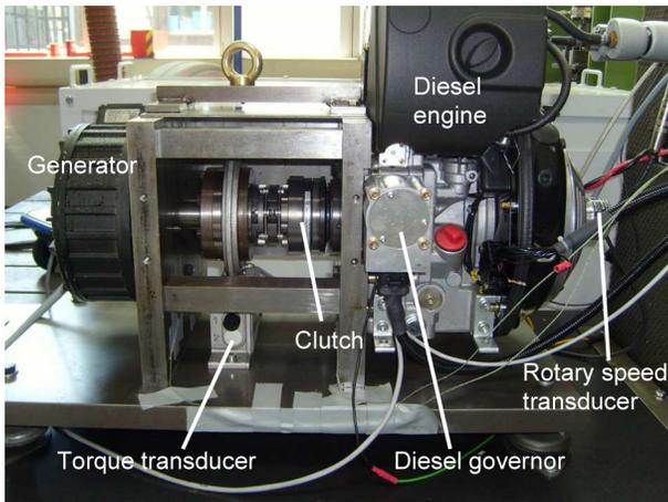
Fig. 6. Test bench with mounted diesel engine and generator
