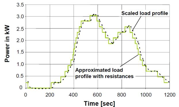
**Fig. 5. Approximation of load profile with resistances**
