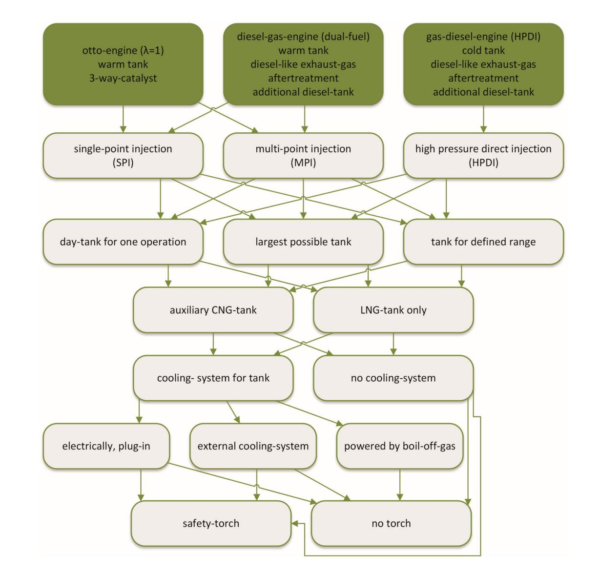
tanks and their surroundings, heat inflow into the tank cannot be avoided. Consequently, constant evaporation of LNG takes place in the tanks, referred to as "boil- off- gas".
